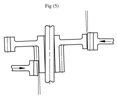
Offset Tooth Loading on Driving & Driven Gears
