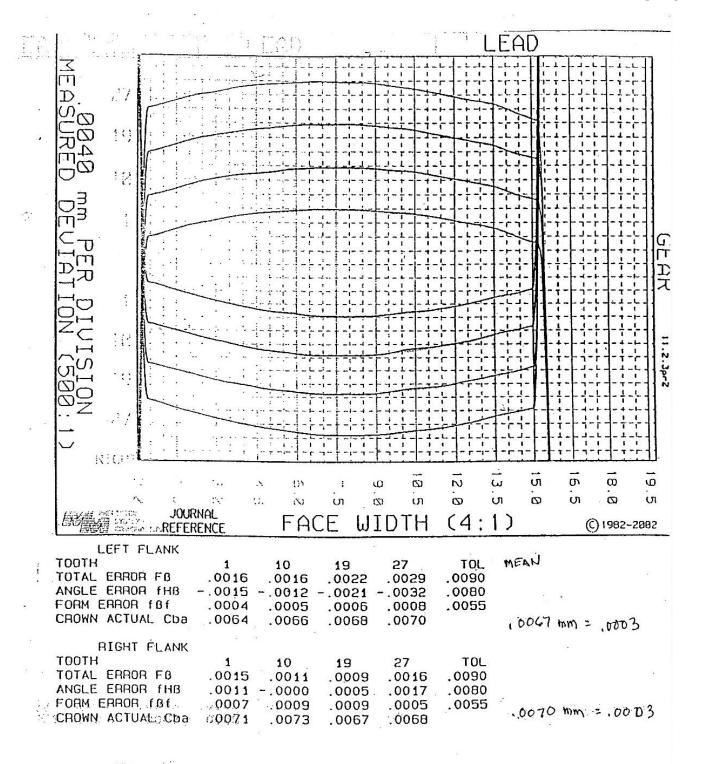
Figure (11) Inspected crown on a machined steel automotive gear
